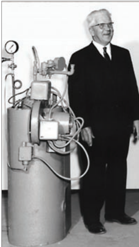
Lewis Palm with his vertical tubeless boiler.
