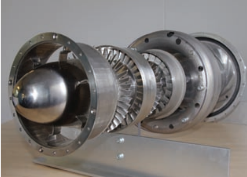
The world's first 3D printed jet engine, created in 2015 at Monash Centre for Additive Manufacturing in Melbourne, Australia.
