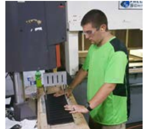
Auburn P-TECH student Will Townsend is ultrasonic welding two pieces of plastic while interning at Bo-Mer Plastics.
