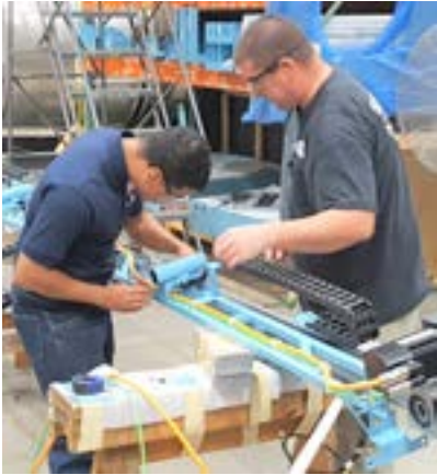
Syracuse P-TECH student Travius Berkley works with mechanical assembler, Brock Nason, while interning at G.A. Braun. He is assembling a spread rail assembly for a sheet feeder. The machine feeds bed sheets into an ironer.
