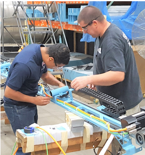
Syracuse P-TECH student Travius Berkley works with mechanical assembler, Brock Nason, while interning at G.A. Braun. He is assembling a spread rail assembly for a sheet feeder. The machine feeds bed sheets into an ironer.
