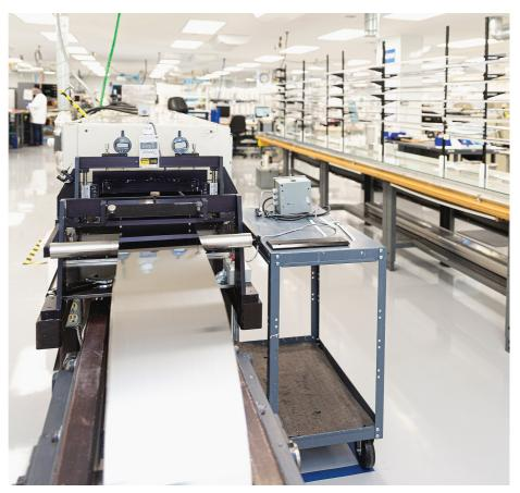
A tape casting machine is ready for the next run.
