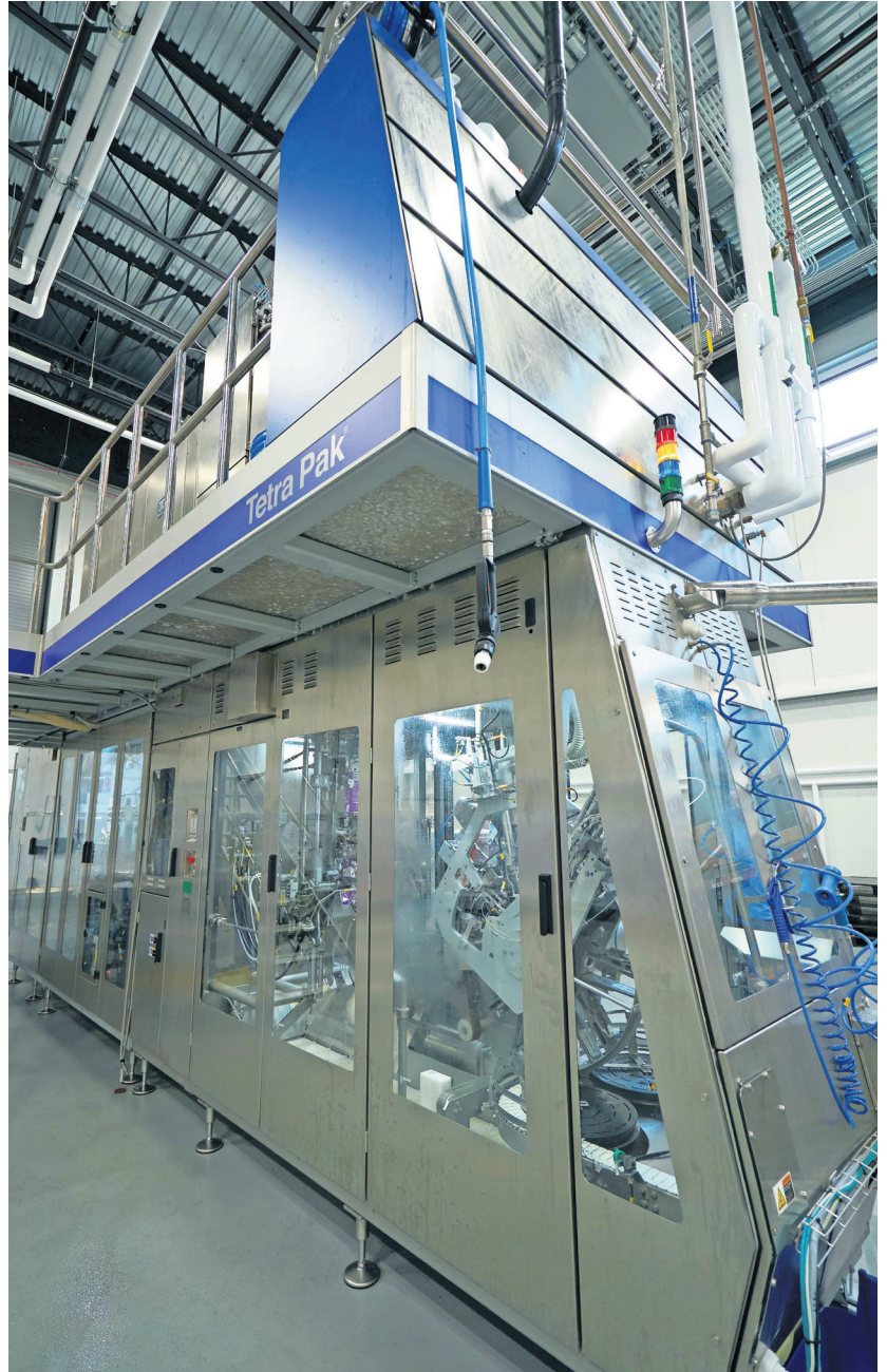
An aseptic filling machine at Byrne Dairy, Inc. CHUCK WAINWRIGHT
